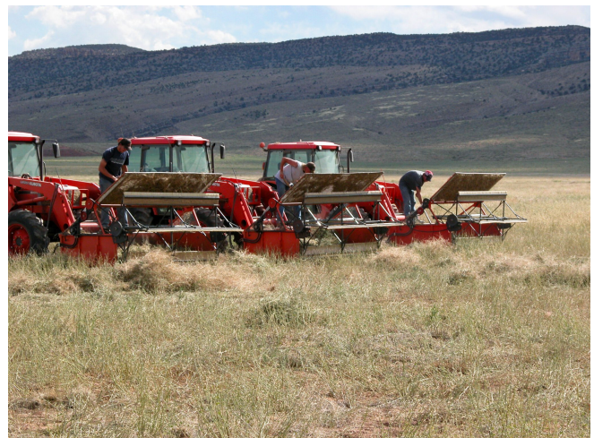
Figure 9. Strippers with hoppers used to mechanically harvest dense small-leaf globemallow stands growing near the Utah-Arizona border. Photo: S. Young, USU.
